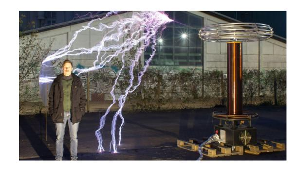
Resonant frequency of this tesla coil is 40kHz, that makes it more dangerous. Also arcs this size can cause serious burns.
